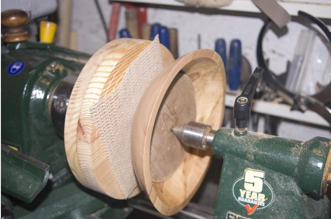
Above shows my flat faceplate and some anti-slip matting you can buy from caravan stores. The faceplate is made from some ordinal pine planks, glued at right-angles to the grain for rigidity and strength. The scroll-chuck holds onto another piece of wood glued and screwed again, across the grain. The whole thing was turned to about 10" diameter. You can see in the photo that I have marked with a point-tool radiuses every 10mm, making it easy to make sure the piece of work is centralised.
