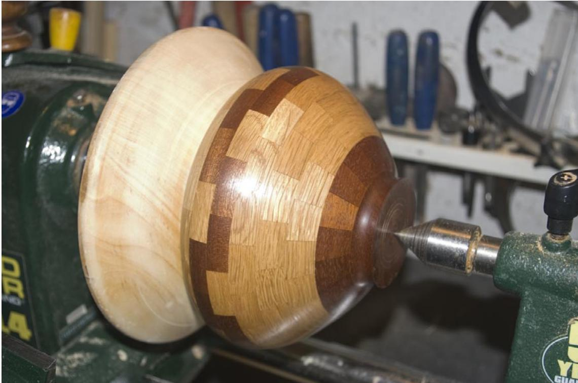
The cone is a simple flat-sided cone of about 10" diameter. It has a recess on the back which fits my scroll chuck, so it is held firmly. Being a straight cone means it will fit most openings of hollow forms and bowls which are not too shallow. It is automatically self-centering. As my segmented bowl is fitted in the picture, you can see that I have plenty of room to finish the foot of the bowl.
